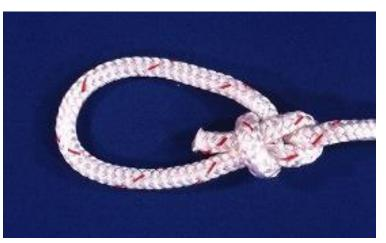
A bowline knot, the knot most commonly used by parasailing operators in their towlines. This type of knot can weaken a brand-new rope by as much as 70 percent.
