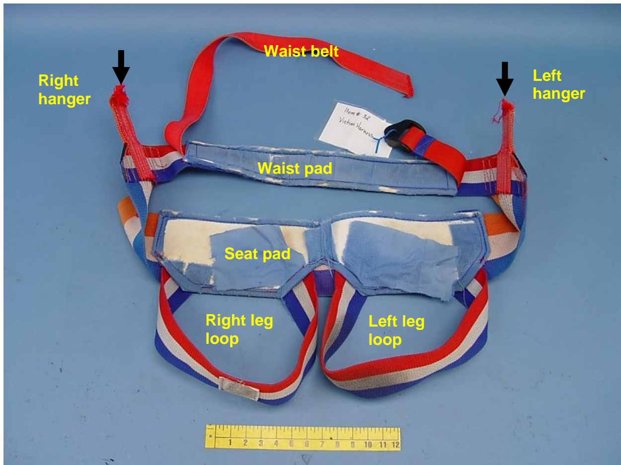
Figure 7. Fractured harness, worn by the victim. The black arrows illustrate the fractured ends of the hangers.
