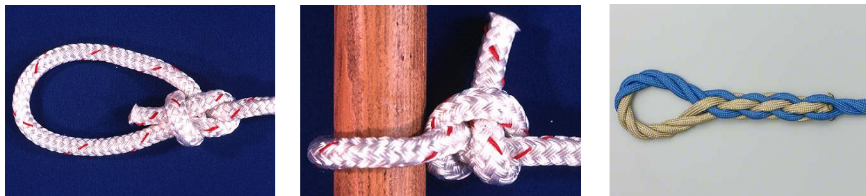
Figure 3. The photos illustrate three ways to fasten a rope: A bowline knot (the most commonly used knot in parasailing operations); a hitch knot; and a spliced eye. (Bowline and hitch knot photos by James Aber; spliced eye photo by Grog, LLC.)
